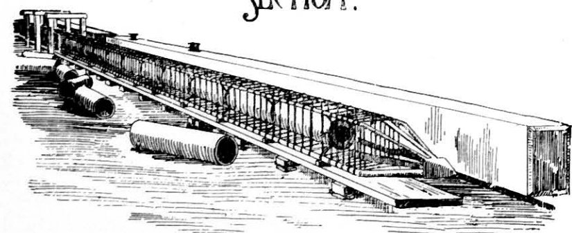
STEEL SKELETON &amp; FINISHED PILE.
