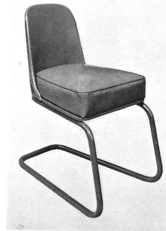
S.G. 4009. Control Chair in tubular steel, upholstered in grey rexine. The chair-back is reinforced with steel straps between padding. The exposed surfaces of metal are stove enamelled
