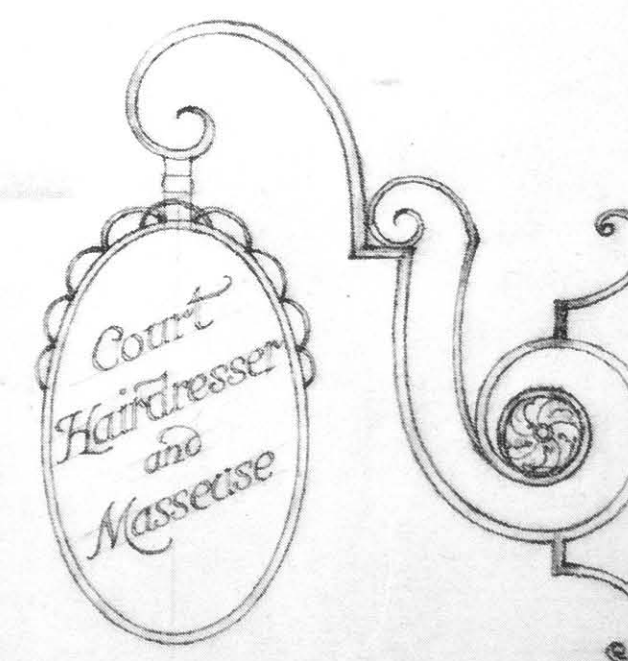
WROT IRON BRACKET WITH BRONZE & ENAMEL SIGN N o S. G. 7004
