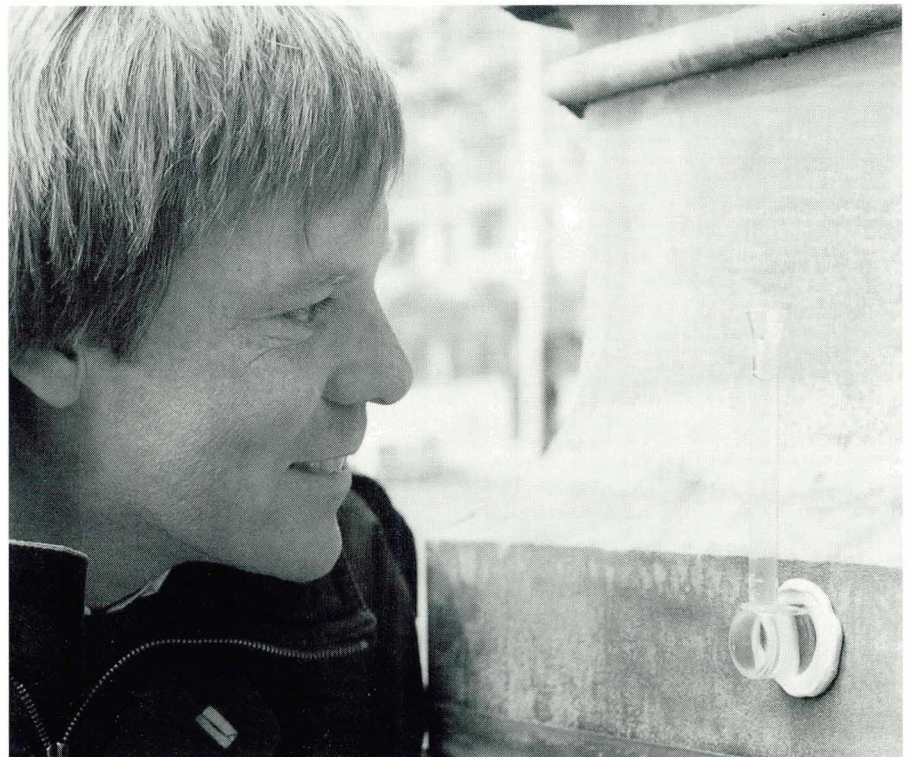
Plate 6.1 Measuring water absorption rate.
