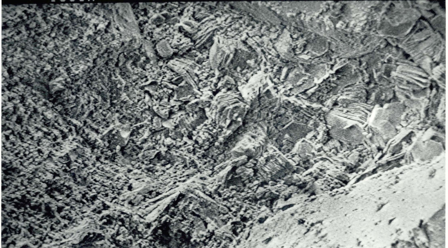
Plate 4.10 SEM photomicrograph of Cat Castle Sandstone after cleaning by dry grit blasting at 80psi. The clay minerals to the left (kaolinite) have been pulverised by impact and there is a lot of debris on the stone surface.
