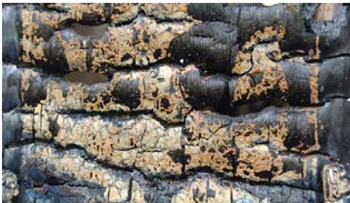
Illus 3 This charred timber door panel, illustrates the destructive and irreversible nature of fire
