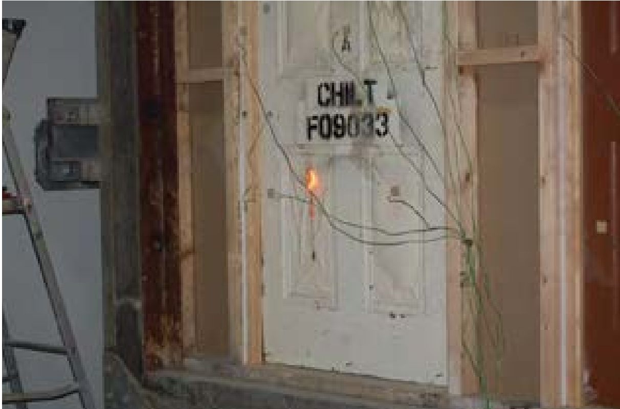
Illus 34 Fire initially attacks areas of weakness as seen in this furnace test where the thin door panels have failed early in the test
