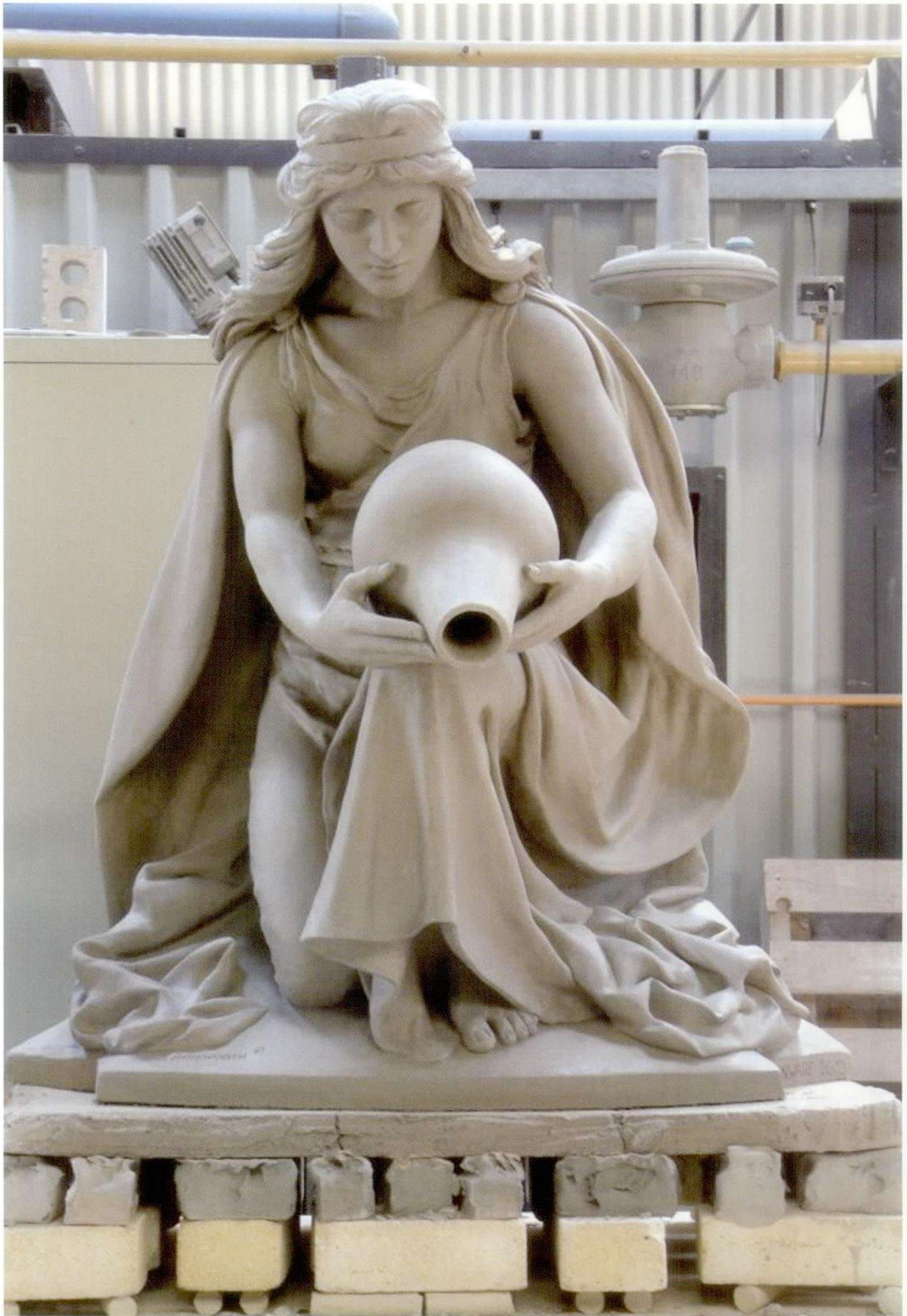
The finished sculpture of Water Bearer No. 3 dries out on a sacrificial base and multi directional rollers designed to control drying-out shrinkage.
