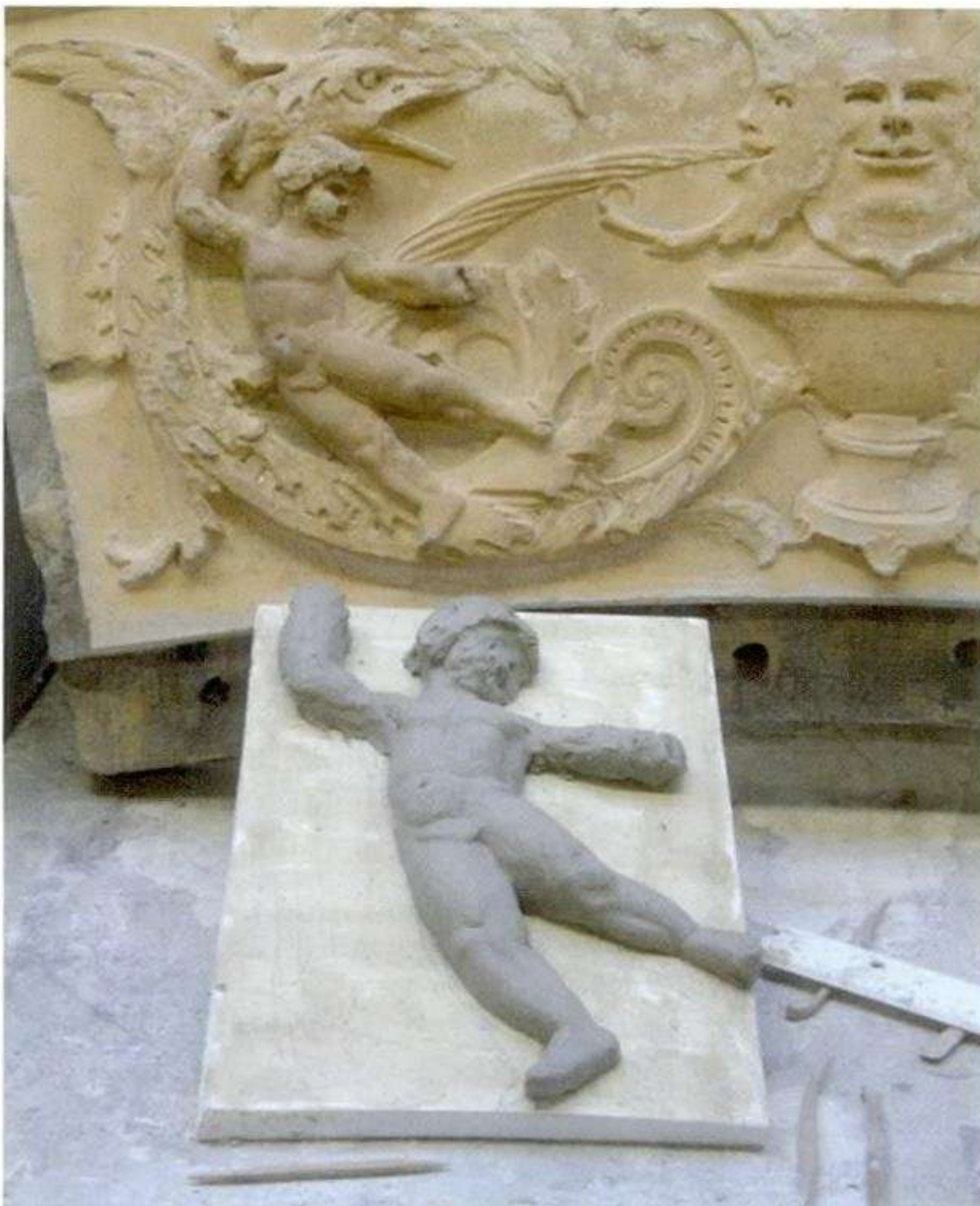
Making moulds of the decorative blocks required close study of the original piece. The decorative elements were made by the sculpture modeller and applied to the base shape prepared by the model makers. (All: Ibstock Hatherware)
