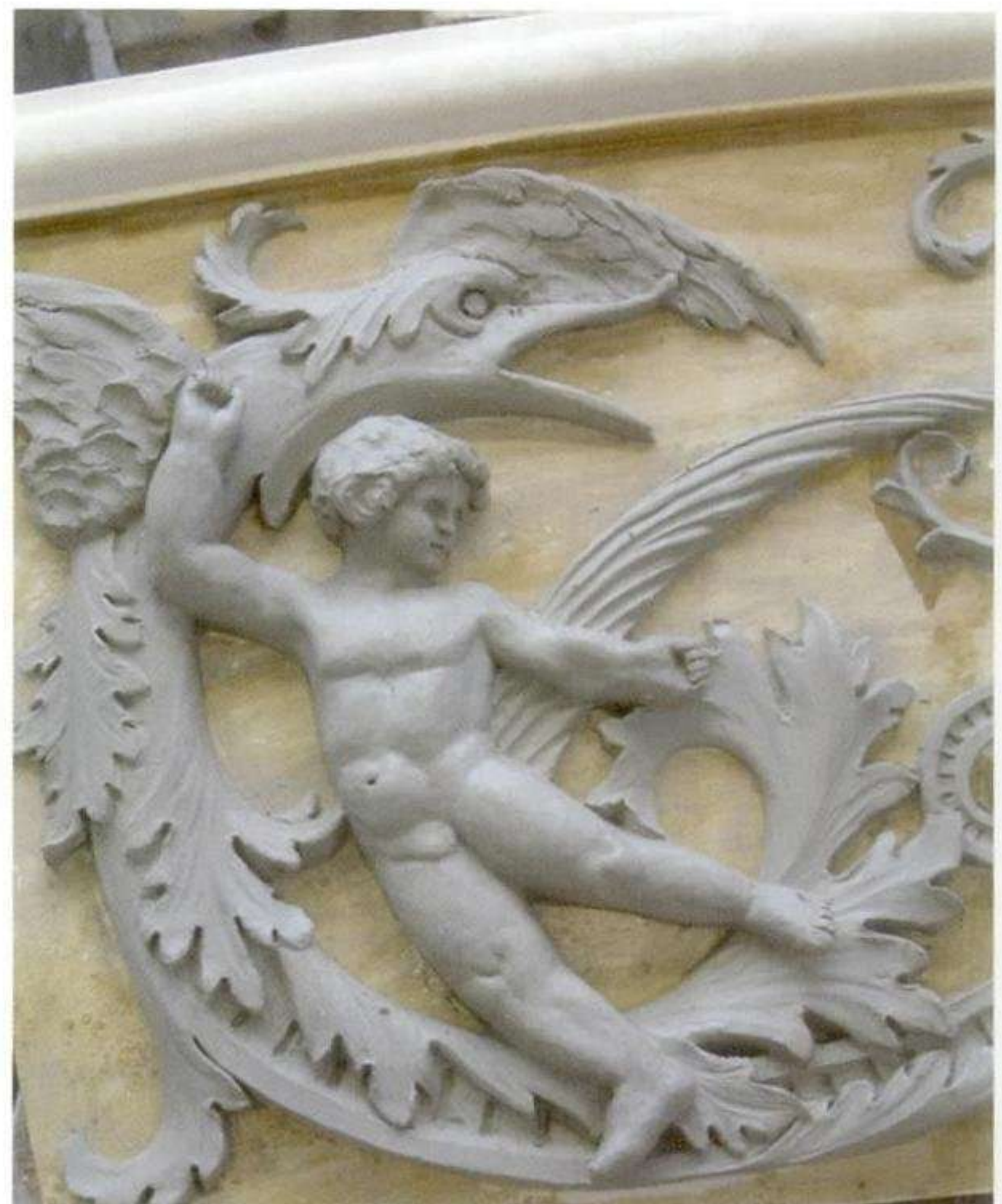
Making moulds of the decorative blocks required close study of the original piece. The decorative elements were made by the sculpture modeller and applied to the base shape prepared by the model makers. (All: Ibstock Hatherware)
