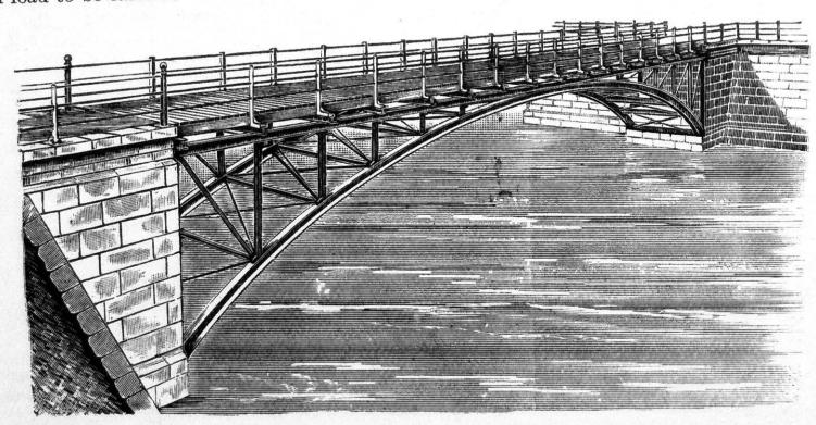
Design No. 570 shows an Arched Bridge of light and elegant appearance. This type requires very strong and substantial abutments, and where these can be cheaply built it will form an economical Bridge, and is particularly to be recommended where appearance is an object. It may be made in spans up to 200 feet or over.
