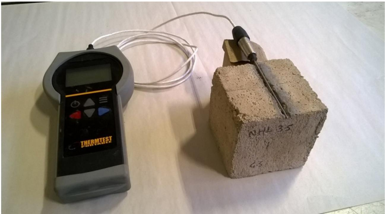
**Figure 5** - Thermtest TLS-100 thermal conductivity probe located in a groove in the face of a specimen.
