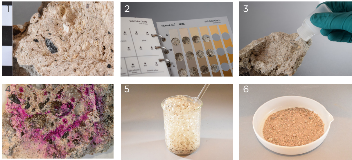
Figure 1 - Different stages of the standard analysis process. 1. visual analysis, 2. colour analysis, 3. testing with Phenolphthalein indicator, 4. pink staining on uncarbonated lime sample for reaction with Phenolphthalein indicator, 5. reaction with Hydrochloric Acid (binder dissolution), 6. Residual aggregate, ready for grading.
