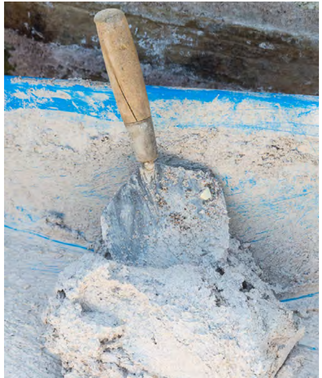
Figure 28: Made from burning limestone, chalk or shells, lime is mixed with water and aggregate to form a workable material.
