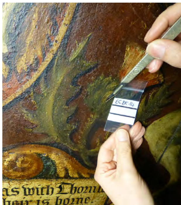
Figure 40: Taking a paint sample at Edinburgh Castle. Paint sampling methodologies are not always undertaken consistently.
