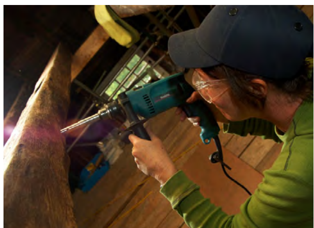
Figure 65: Dendrochronology analysis being undertaken at Newark Castle. Limited recording and analysis of timber is currently undertaken.
