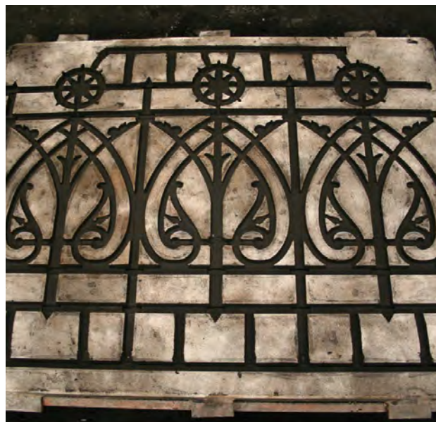
Figure 26: Cast iron railing mould for a design found in Stornoway, Isle of Lewis. The number of architectural pattern makers and moulders working in Scotland is limited.
