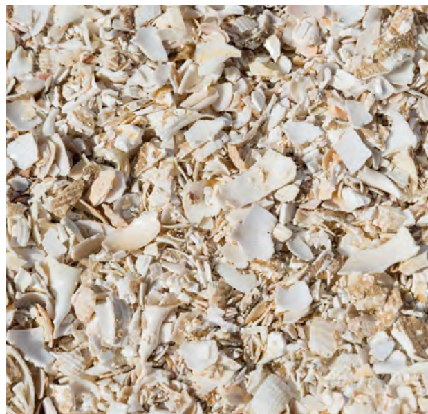
Figure 34: Different lime products and aggregates can be used to tailor specifications to reflect regional variations or achieve performance requirements, but can be challenging to access. Crushed shells were used for repairs to walls at Kinneil House.
