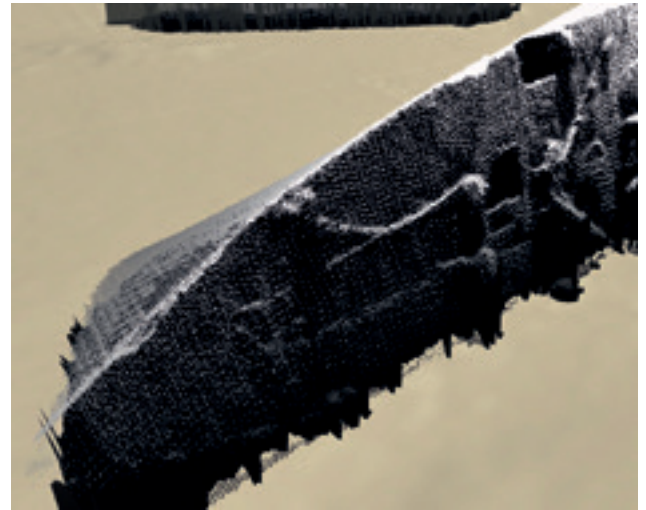
Point cloud of individual multibeam soundings from the wreck of the German escort vessel F2 in Scapa Flow. The huge increase in marine survey capabilities over the last two decades requires effective strategies for handling and storing very large data sets. Image © Crown Copyright, Historic Scotland – image produced by Wessex Archaeology.
