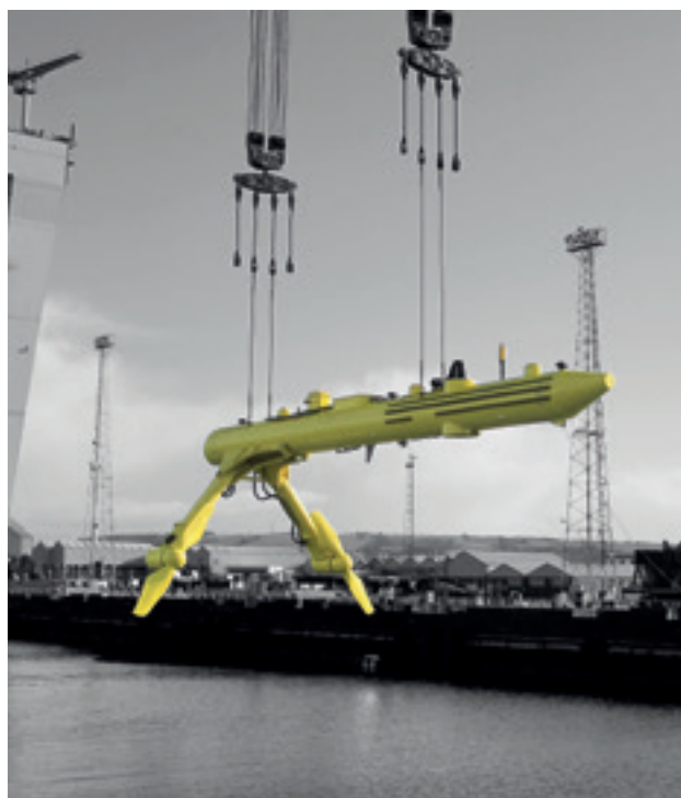
The SR250 has two tidal stream turbines mounted beneath a hull that floats at the surface and is tethered to the seabed. Image © Scotrenewables Tidal Power Ltd.
