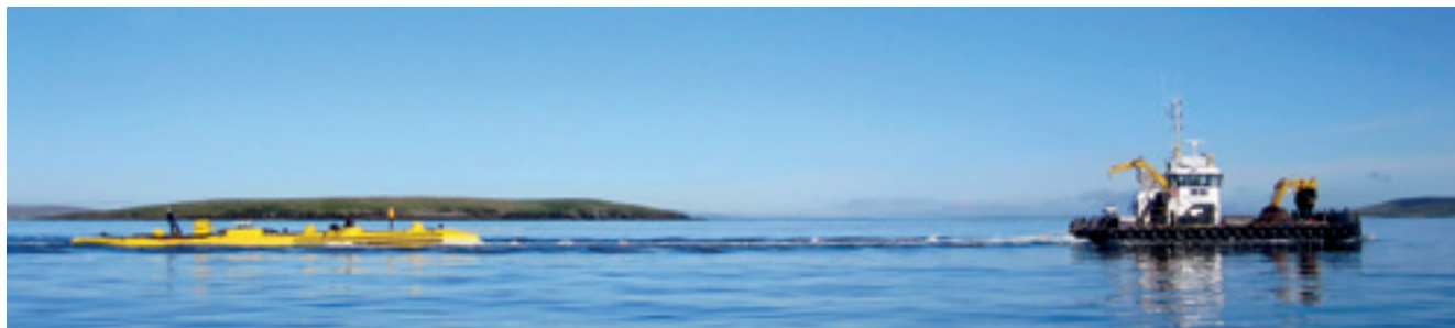
Devices such as the SR250 that are tethered to the seabed can be removed for maintenance using relatively small vessels. Image © Scotrenewables Tidal Power Ltd.
