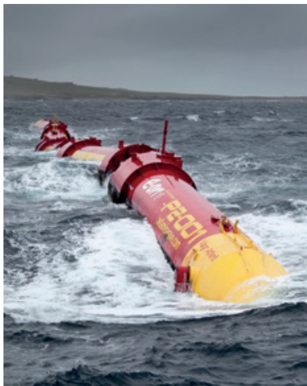
The Pelamis is a wave device that floats on the surface and is tethered to the seabed. It is designed to operate in relatively deep water offshore. Image © Pelamis Wave Power.
