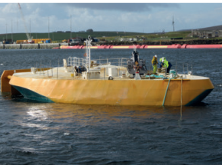
Wello Penguin: a wave device tethered to the seabed. Image © Wello.
