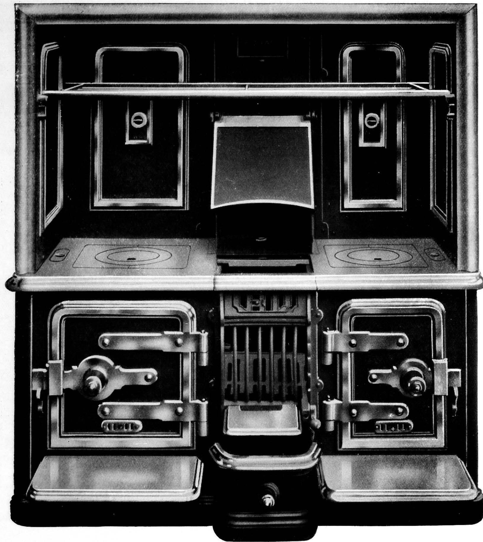
No. 15.—"THE CHAMPION" RANGE, with strong sheet-iron ovens, bright hinges, bracket shelves, "Eagle" lifting fire with wrought-iron bars and cast fall bar, with ashpit linings, ashpan, 2 in. round corners, jamb bead, iron covings and covering-in plate, platerack, bright mounted.
