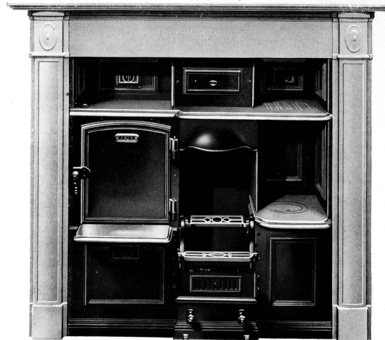
No. 55.—YORKSHIRE RANGE, with projecting platerack, cast sectional oven, corrugated bottom, plain raised oven door, saddle to protect bottom and corner of oven next fire, "Renown" barless fire with reversible top trivet, bottom trivet nickel-plated, slow combustion arrangement to fire, ashpan, G. and B.B. canopy to fire, projecting hob, coves, 2-piece swing smoke slip, bright O.G. mouldings, black panel mouldings, building strips added.
