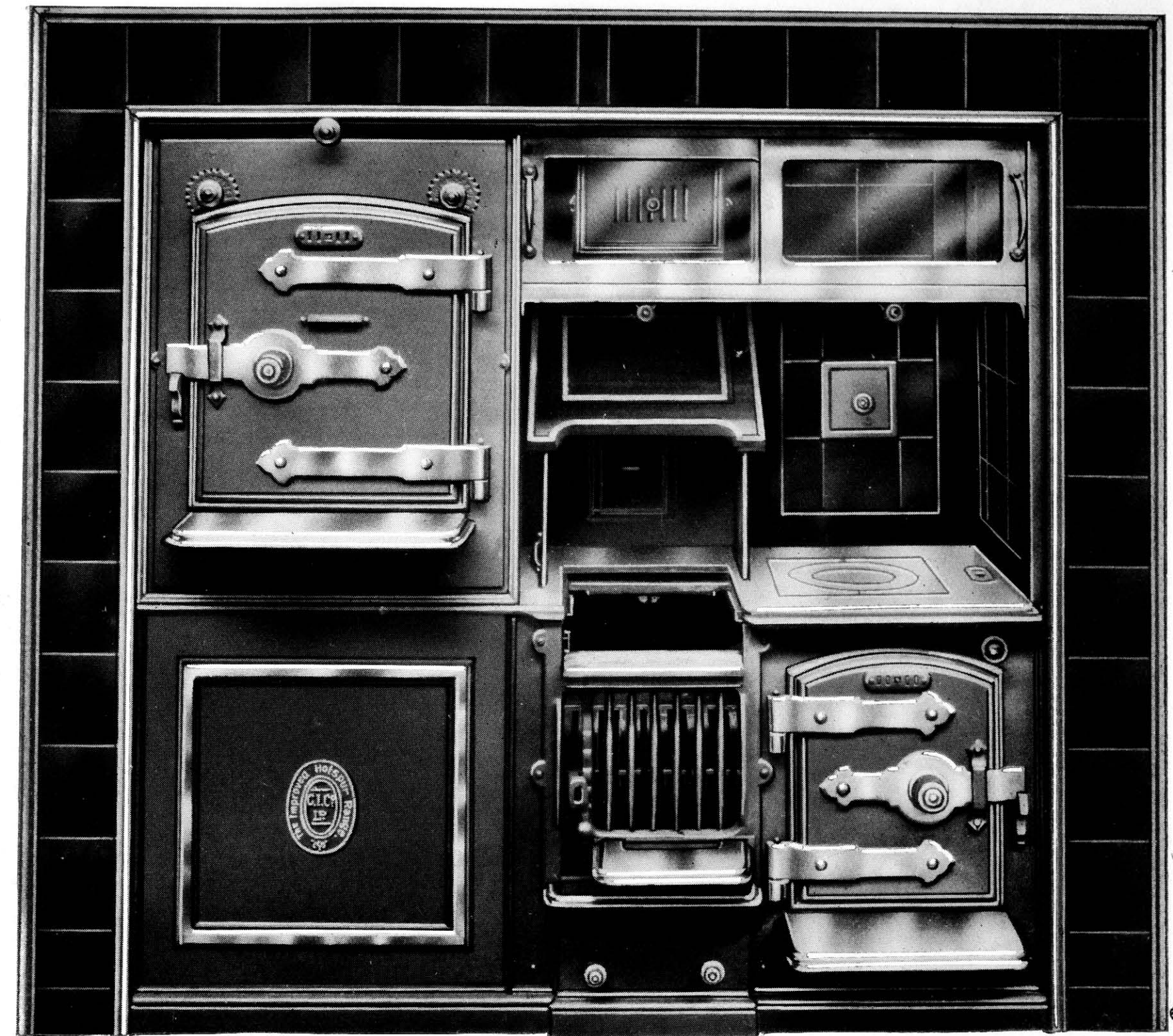
No. 10.—IMPROVED "HOTSPUR" RANGE, open and close fire, with high baking oven and low roasting oven, both ovens of strong sheet-steel, baking oven fitted into brick lined casing, removable from the front, and provided with cast-iron flues, roasting oven with double crown and extended panelled hotplate, "Eagle" lifting fire with steel bars, bottom trivet, ashpan with cinder grating, slow-combustion arrangement, and with back plate and damper for pressure boiler, tiled covings, cast plate-rack, hot closet with sliding doors with glass panels, covering-in plate, and the whole surrounded by polished mouldings fitted with 6x6 in. tiles. Stove dried Berlin black finish with bright mountings.
