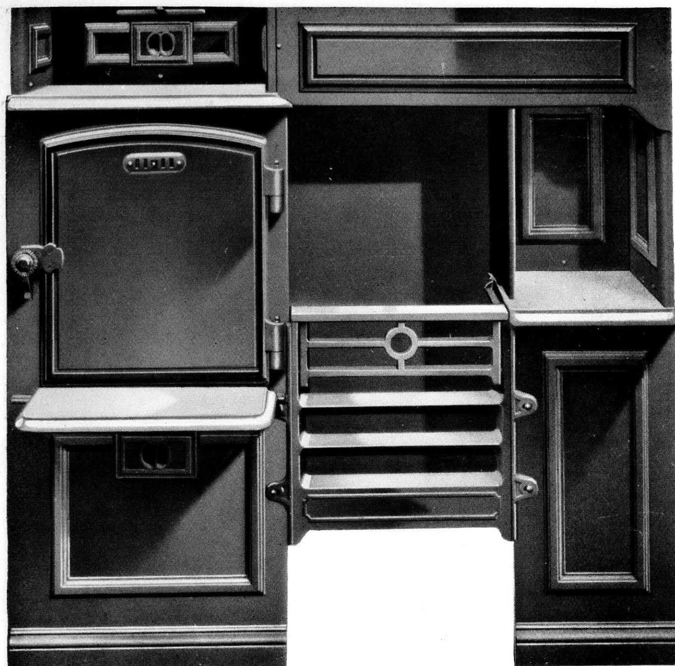
No. 16 A.—YORKSHIRE RANGE, with cast sectional oven, corrugated bottom, plain raised oven door, bright bracket shelf, saddle, strong cast bars and fall bar, coves and 2-piece swing smoke slip, bright O.G. mouldings, black panel mouldings and fall bar, long archplate.
