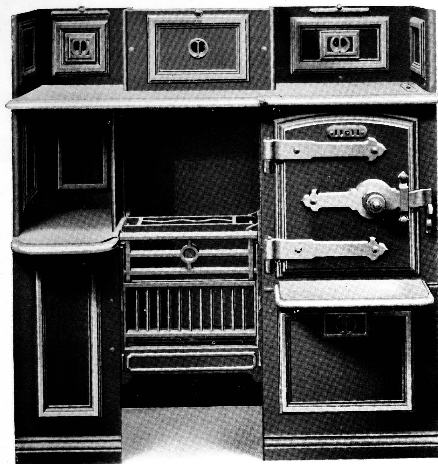
No. 39 A.—"UMBRIA" RANGE, with projecting platerack, cast sectional oven with corrugated bottom, hollowtop, raised oven door, saddle to protect bottom and corner of oven next fire, steel sliding bars and fallbar, fallcove, projecting hob, cove 2-piece swing smoke slip, bright O.G. mouldings, black panel mouldings and fallbar, building strips added.
