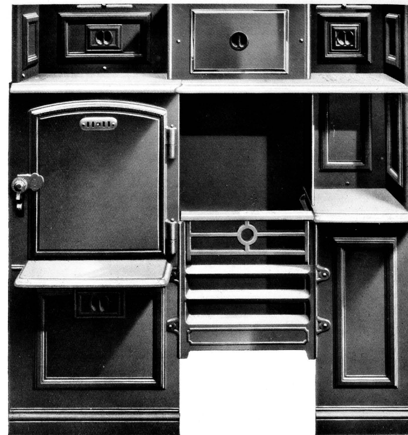
No. 17 A.—YORKSHIRE RANGE, with projecting platerack, cast sectional oven, corrugated bottom and saddle, plain raised oven door, strong cast bars and fall bar, 2-piece swing smoke slip, black panel mouldings and fall bar.
