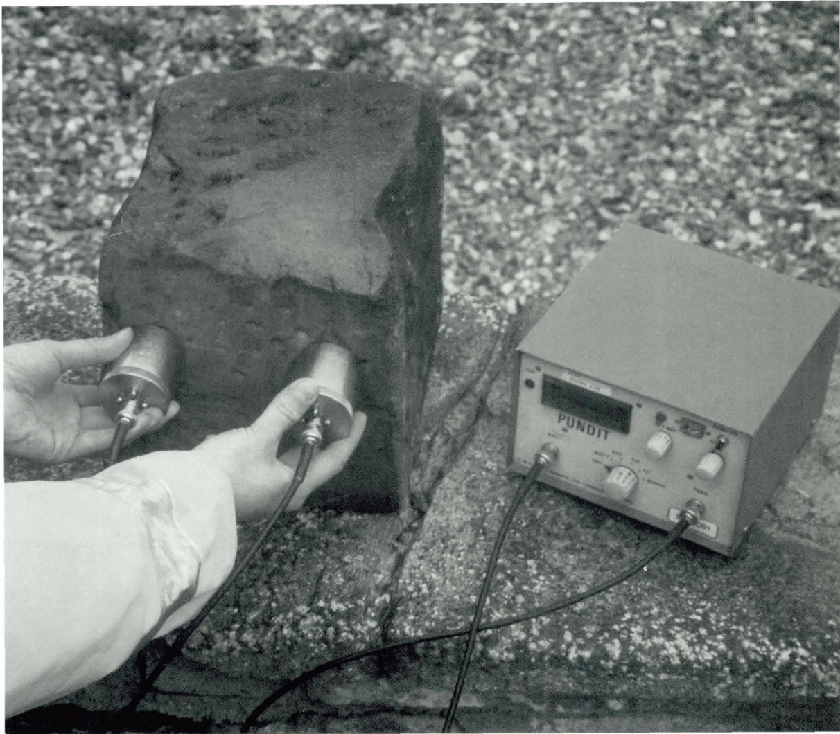
Plate 9 Typical UPV survey in operation (indirect arrangement of couples both on the same side of the object being tested)
