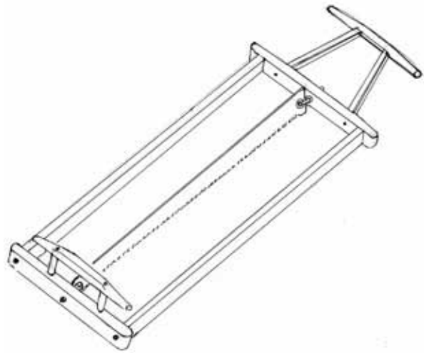
Illus. 26 Pit sawing on a trestle or in a pit (BW)
