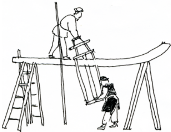
Illus. 25 Sawing on a saw horse (BW)
