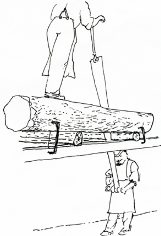
Illus. 27 How timber was sawn a) a log, b) with sides axed away, c) two rip saw cuts producing 2 sile blades and a central section that could be used elsewhere (BW)
