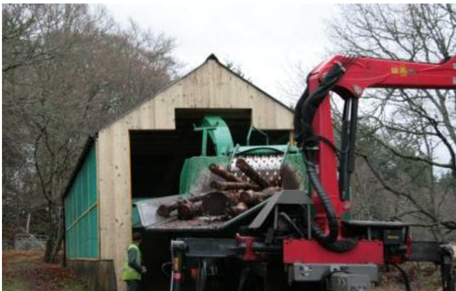
Fig 5: Logs being processed by wood chipper
