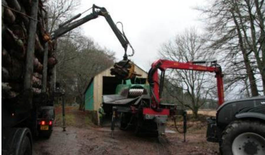
Fig 4: Crane on lorry loading SRW logs into the wood chipper
