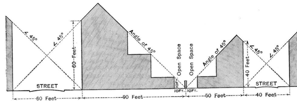
Fig. 725.—Diagram illustrating Regulations for New Houses in Liverpool.
