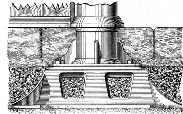
Fig. 728. — "Self-fixing" Base for Cast-iron Stall-pillar.
