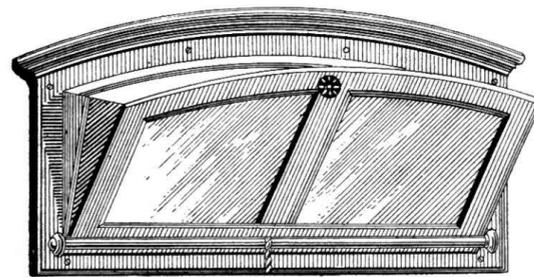
Fig. 735.—Combined Window and Air-inlet.
