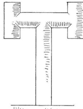
Fig. 690.—Chimney-cowl of Sheet Iron or Steel.
