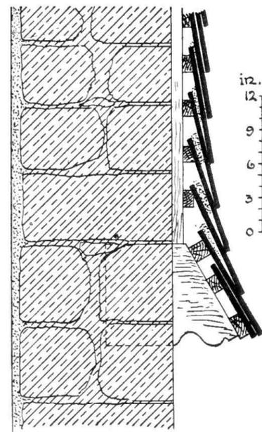
Fig. 682.—Section showing a Method of Covering an Old Wall with Weather-tiles.
