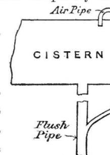
Fig. 666.—Faulty Connection of W.C. Flush-pipe and Cistern.
