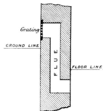
Fig. 668.—Air-flue for Ventilating Floor below Ground.
