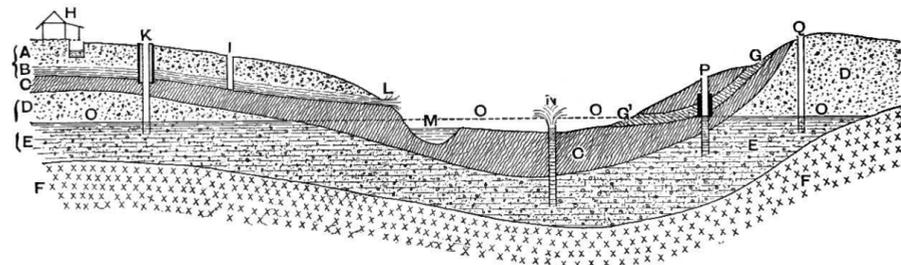
Fig. 726.—Diagram showing ground-water, deep water, spring, stream, and different kinds of well:—
