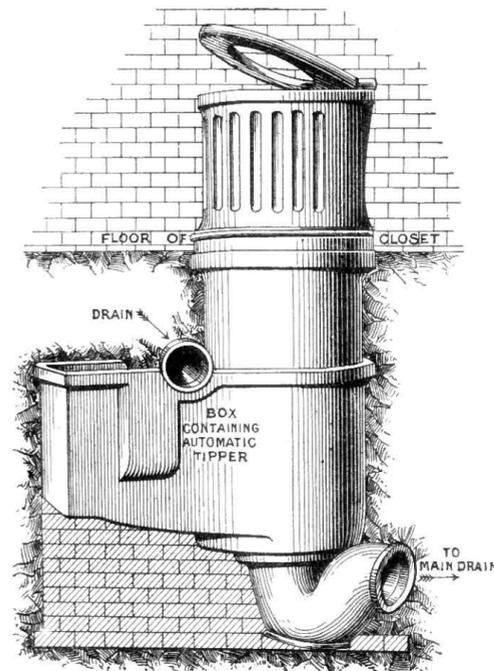
Fig. 704.—View of Duckett's Slop-water Closet.
