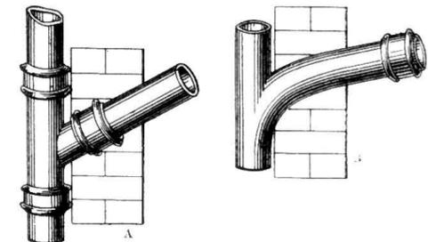
Fig. 699.—A, Faulty; B, Satisfactory Connection of Closet-outgo with Soil-pipe.
