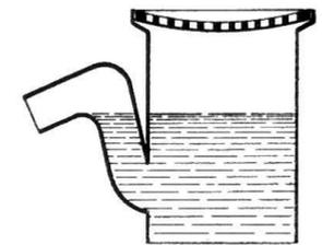
Fig. 670.—Section of Old-fashioned "Cesspool" Gully.
