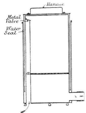
Fig. 673.—Section of Smoke-machine for Testing Drains. a, Perforated tray for cotton waste.
