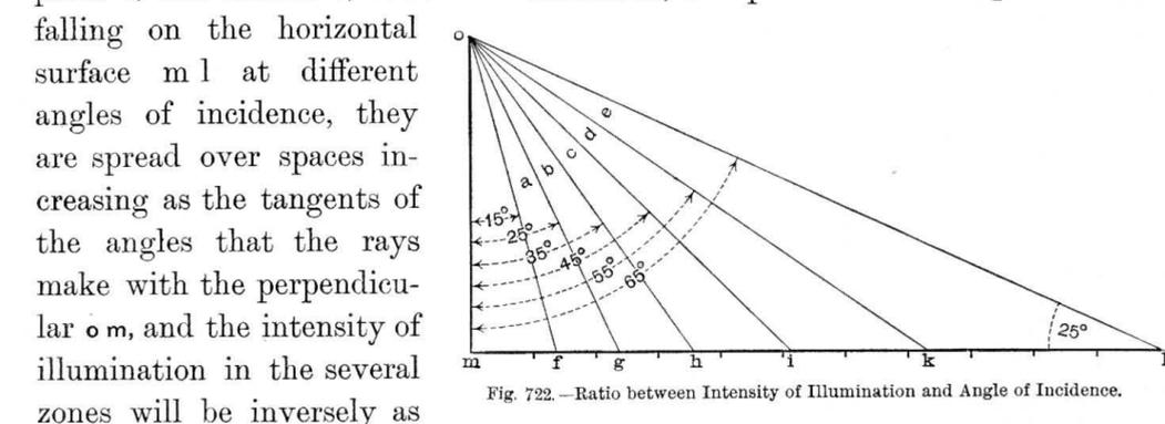
Fig. 722.—Ratio between Intensity of Illumination and Angle of Incidence.
