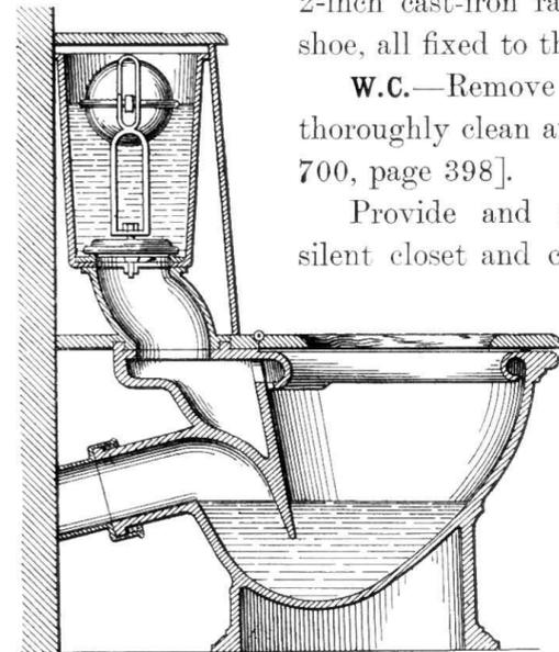
Fig. 707.—Section of Shanks's Combination Silent Closet and Cistern.
