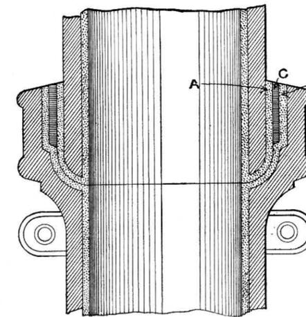
Fig. 743.—Brighton and Venning's Patent Lead-lined Iron Pipe.
