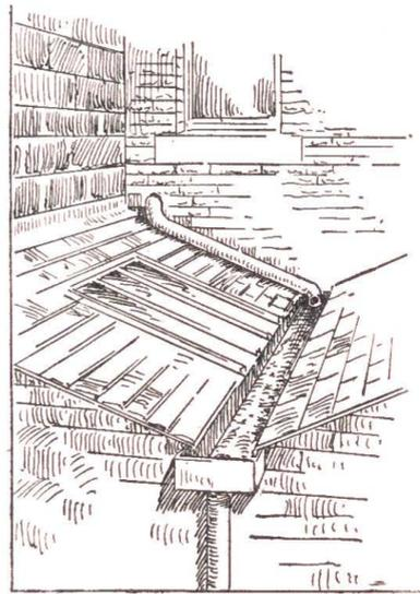
Fig. 700.—Dangerous Soil-pipe and Soil-gutter, actually found by the writer in an existing house.
