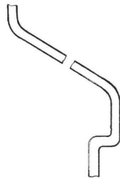
Fig. 674.—Faulty Outlet-shaft for Drain-ventilation.
