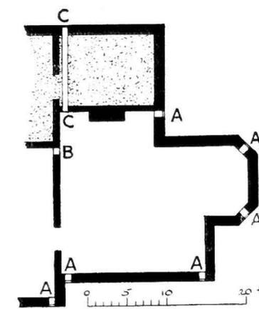
Fig. 683.—Plan showing Ventilation of Space under Wood Floor.
