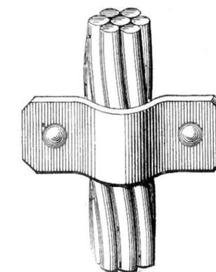
Fig. 713.—Half-inch Copper-rope Lightning-conductor, composed of 7 wires.
