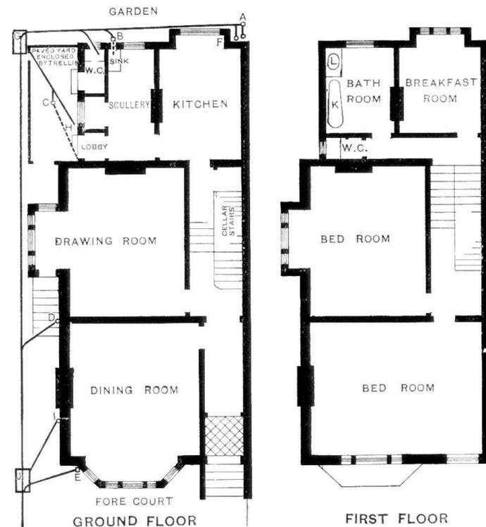
Fig. 698.—Corrected Sanitary Arrangements of a Suburban Villa.
