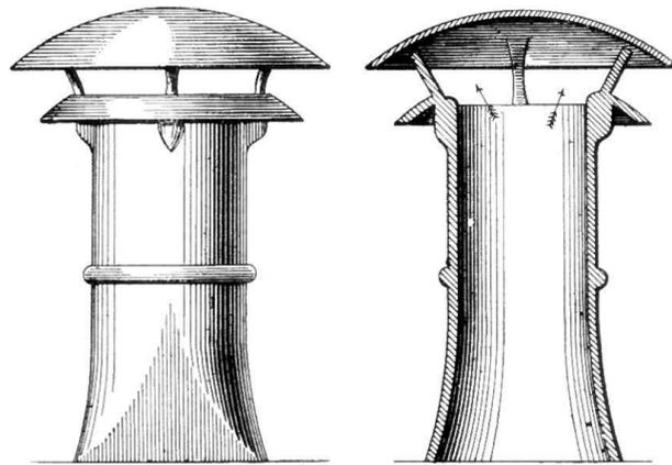
Fig. 687.—Elevation and Section of the Pembridge Chimney-cowl.
