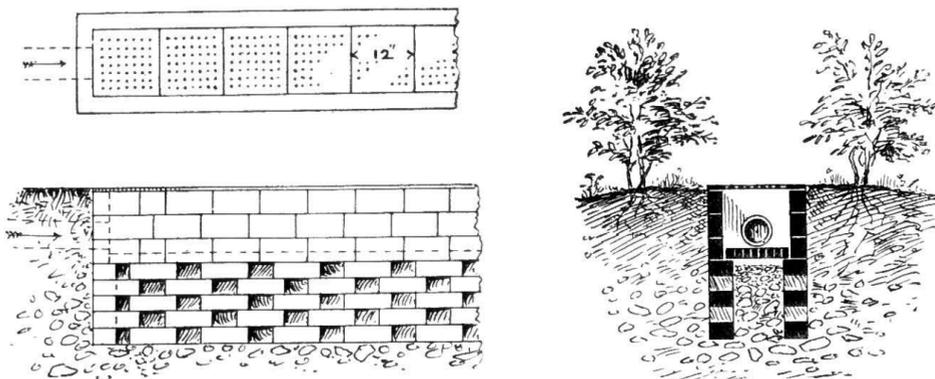
Fig. 709.—Plan, Section, and Elevation of Filtration-gutter.
