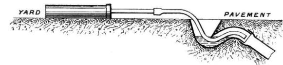
Fig. 671.—Sheath and Tubes for Smoke-rocket.
