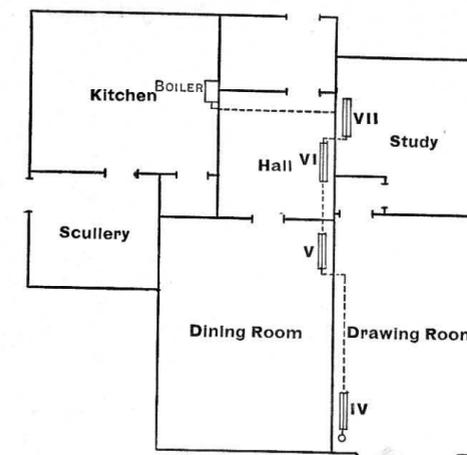
Fig. 746.—Ground-floor Plan of House warmed from Kitchen-boiler.
