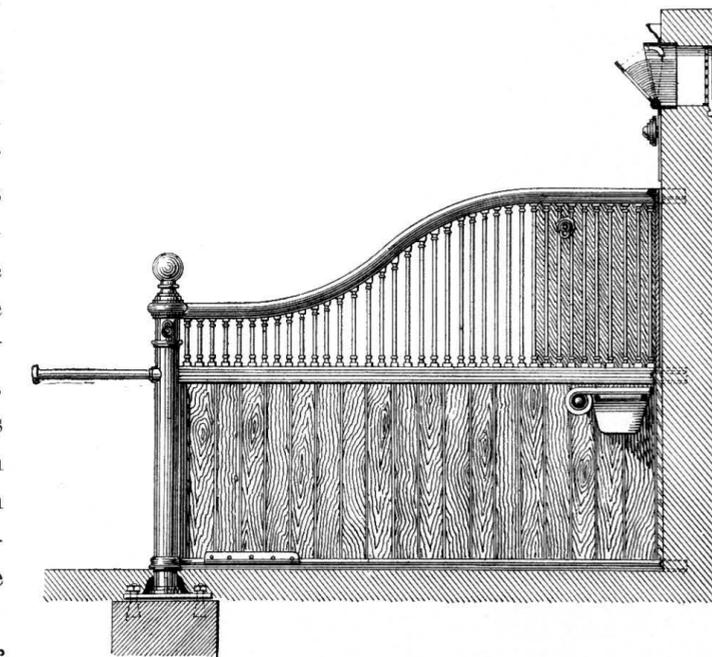
Fig. 729. — Stall-division with Shifting-piece in Sill for taking out and replacing the Woodwork.
