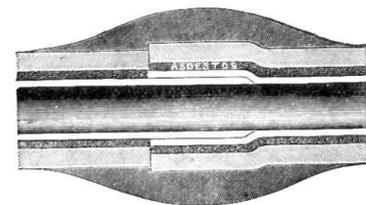
Fig. 693.—Straight-joint in the "Eureka" Tin-lined Lead Pipe.
