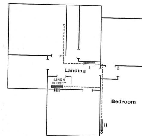
Fig. 747.—First-floor Plan of House warmed from Kitchen-boiler.
