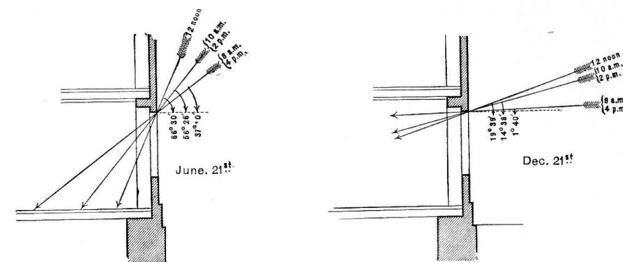
Figs. 720 and 721.—Incidence of the Sun's rays at Noon in Window facing South between the hours of 8 a.m. and 4 p.m.
