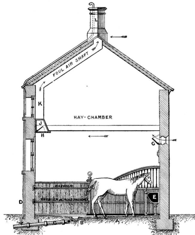
Fig. 730.—Section through Stable and Hay-loft, showing Drainage and Ventilation.
