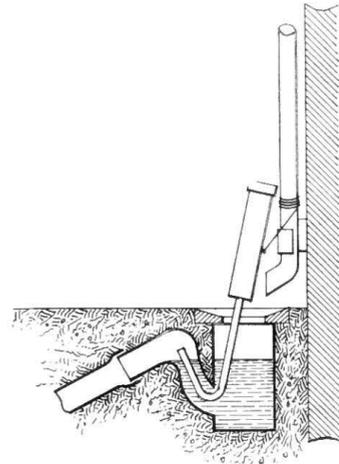
Fig. 672.—Sheath with Bent Brass Tube for Smoke-rocket.
