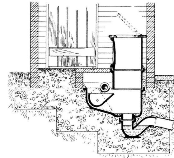
Fig. 703.—Section of Duckett's Slop-water Closet.
