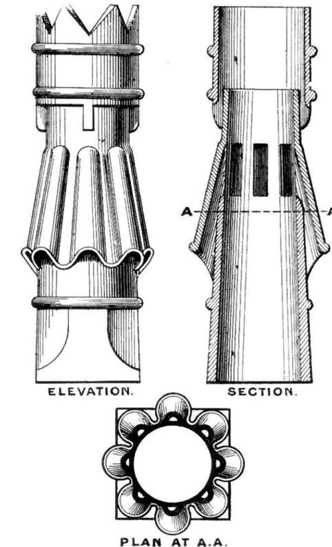
Fig. 689.—Elevation, Section, and Plan of the "Success" Chimney-pot.
