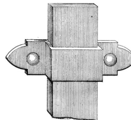
Fig. 712.—Sanderson's Copper-tape Lightning-conductor, 1 in. +  $\frac{1}{8}$  in.
