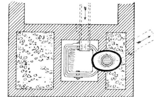
Fig. 702.—Plan of Duckett's Slop-water Closet.
