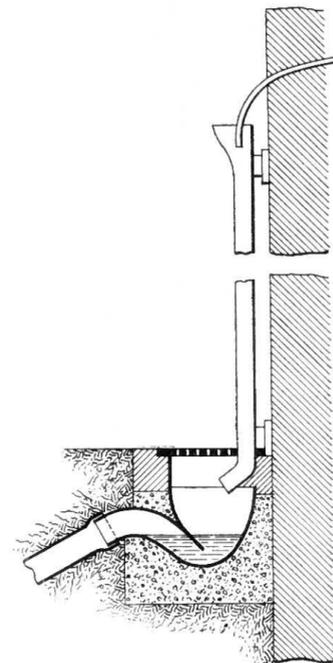
Fig. 669.—Waste-pipe discharging over External Pipe disconnected at Foot.
