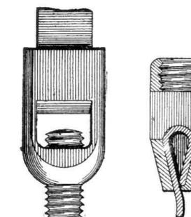
Fig. 715.—Elevation and Section of "the Lewis Link".
