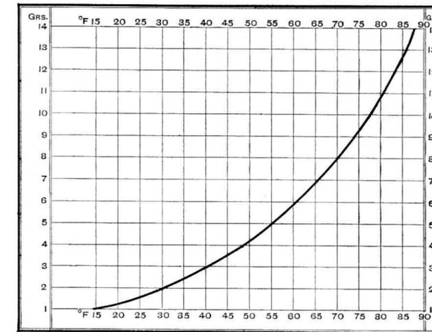
Fig. 716.—Weight (in grains) of water-vapour in a cubic foot of *saturated* air from 15° to 90° F.
