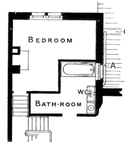
Fig. 705.—Plan of Old Bath-room and W.C.
