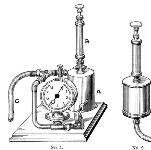
Fig. 749.—The “Jensen” Gas-installation Testing Machine. No. 1, with pressure-gauge; No. 2, without pressure-gauge.
