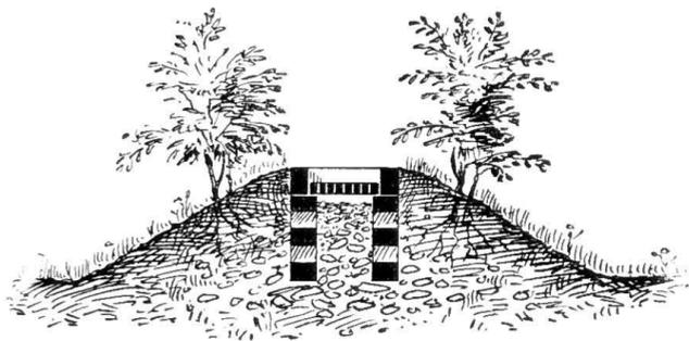
Fig. 710.—Section of Filtration-gutter for Clay Soils.
