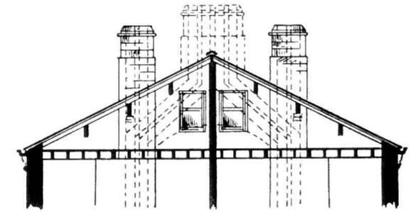
Fig. 686.—Alteration of Chimney-stacks in consequence of insufficient Inclination of Flues.
