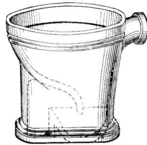
Fig. 697.—View of Defective Wash-down Pedestal-closet.
