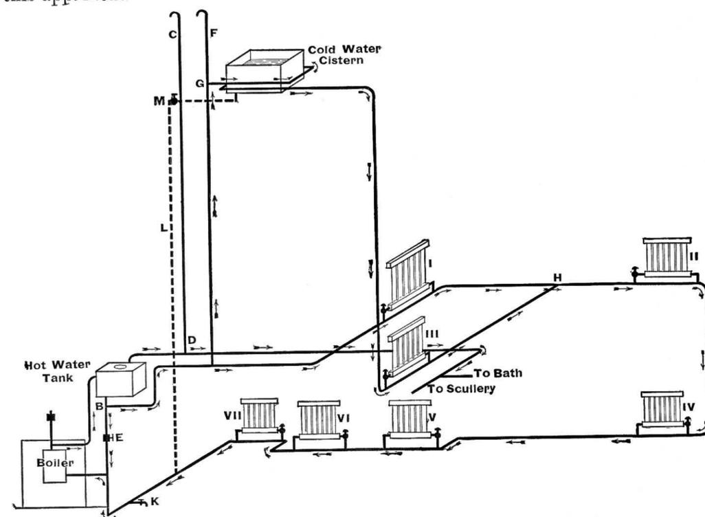
Fig. 748.—Diagrammatic View of Warming Apparatus and Domestic Hot-water Service warmed from Kitchen Boiler.
