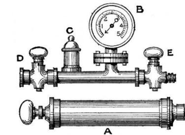
Fig. 744.—The "Jensen" Pneumatic Drain-testing Machine.
