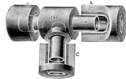
Fig. 694.—Branch-joint in the "Eureka" Tin-lined Lead Pipe.
