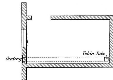
Fig. 676.—Plan of small Bedroom, showing Method of improving Ventilation.
