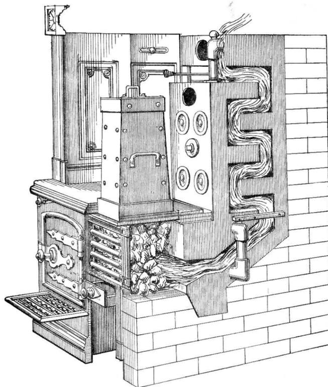
Fig. 745.—Kitchen-range fitted with Potterton's "Zigzag" Boiler and Top-feeder.
