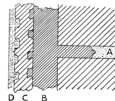
Fig. 681.—Full-size Section of White's Tiles, with Asphalted Cavity for Damp Walls. A, mortar-joint with part raked out; B, asphaltic composition; c, tile; D, plaster.
