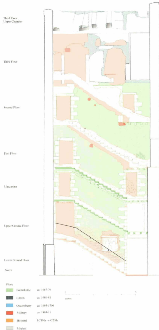
Illus 119 Queensberry House, a sectional elevation through one of the main staircases, with various periods and features recorded into separate CAD layers. ((Drawing: Addyman Associates, courtesy Scottish Executive)
