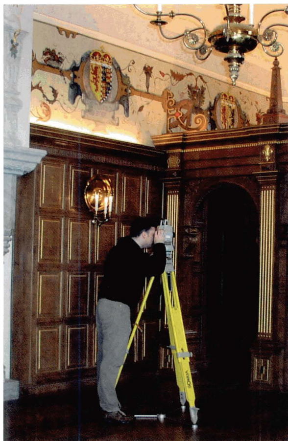
Illus 30 A total station theodolite set up in a historic interior, the Laigh Hall at Edinburgh Castle. While essential for accurate survey control, great care must be taken when using instruments in these surroundings. The tripod 'spreader' to protect floor surfaces can be seen. (Photo: John Gordon/Historic Scotland)
