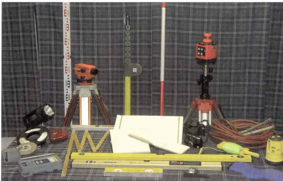
Illus 25 A range of equipment typically used for hand surveying. While the basic tools of tapes and rods are timeless, modern instruments such as the laser level (rear right) can be invaluable in establishing datums. (Photo: Historic Scotland)
