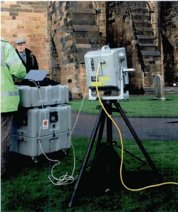
Illus 40 A typical laser scanner instrument, the Cyrax 2500 model, set up in front of part of Dunfermline Abbey. Typically, the instrument is set up between 10 and 20 metres from the façade. (Photo: Ross Dallas)
