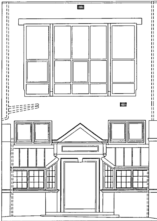
Illus 31 An example of a façade surveyed using a reflectorless EDM instrument. The instrument is set up perhaps 10 to 20 metres from the façade and readings are made directly off the surface. (Drawing: Loy Surveys)
