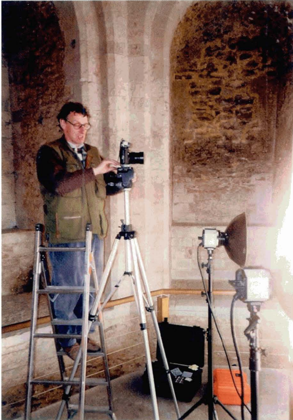
Illus 113 Lighting internal areas or features can be skilled work. In this example, two 'studio' flash heads are being used to provide even illumination of a feature. (Photo: Ross Dallas, courtesy Downland Partnership Ltd)
