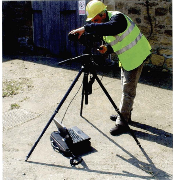
Illus 112 Setting the camera up on a tripod. Use of a tripod will always improve the sharpness of photography and helps with the composition of the photograph. (Photo: Colin Briden)
