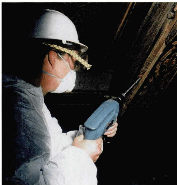
Illus 93 Coring in progress in the Great Hall, Edinburgh Castle. The oak timber has been squared, but the sapwood and sub-bark surface survives on the edge of the timber. The timbers were felled in 1509/10 and came from either southern Sweden or Denmark. (Photo: AOC, courtesy Historic Scotland)
