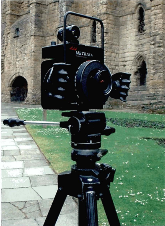
Illus 42 A modern photogrammetric camera, the Linhof 'Metrika', which uses 4 x 5 inch film. This design is based on an existing camera. (Photo: Andrew Morris)
