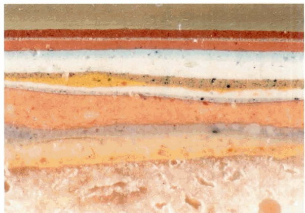
Illus 99 A paint sample cross-section, viewed through a microscope. This sample is from the nave of St Aloysius Church. (Photo: Historic Scotland)
