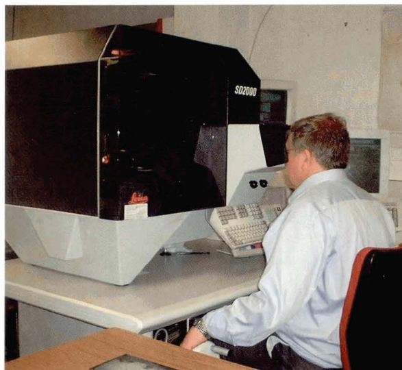
Illus 44 A photogrammetric plotter, the Leica SD2000. This instrument utilises conventional photography on film, but is computer driven. The newest generation of photogrammetric plotters utilise digital imagery. (Photo: Andrew Morris)
