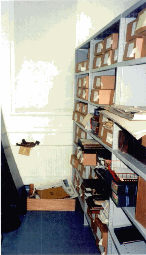
Illus 183 The type of cardboard boxes seen on the racking to the right should not be used for storage, as the material is highly acidic. (Photo : Library Conservation Unit)
