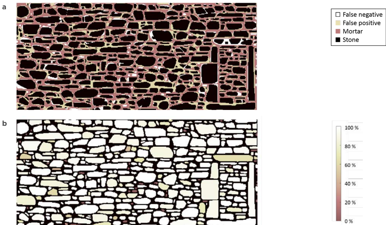
Figures 7a and 7b: Illustration of the assessment of the performance of the proposed wall segmentation algorithm. In a) the labelling performance results are shown. Black and magenta regions are pixels that are correctly recognised as stone and mortar respectively. Yellow regions are 'false positives', i.e. mortar areas that are incorrectly labelled as stone. White regions are 'false negatives', i.e. stone areas that are incorrectly labelled as mortar. In b) each stone is coloured according to the percentage of its area (in the orthophoto) that is properly labelled as stone.
