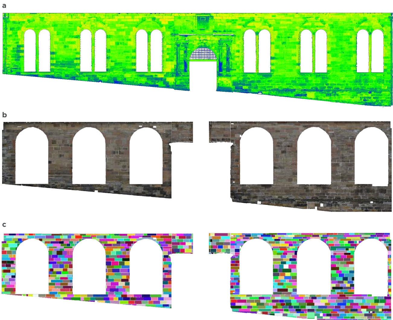
Figure 21: a) Point cloud obtained from terrestrial laser scanning; b) Point cloud coloured with photogrammetry RGB values; c) Segmented ashlar point cloud.
