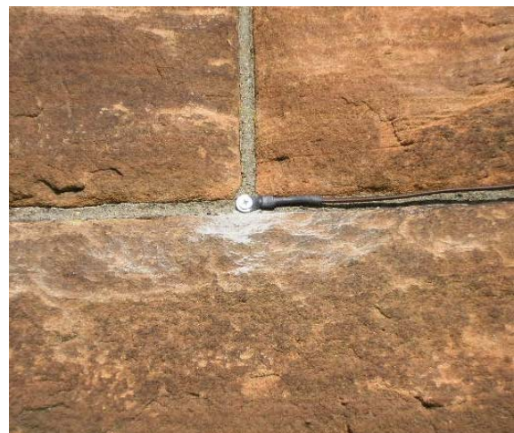
Figure A7: Method of mounting external surface temperature sensor to mortar joint not made where access was a problem, or fixing in the manner described would damage the external finish.
