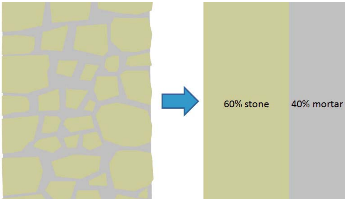
Figure 5. Traditional solid wall construction: the left figure (a) shows a schematic diagram of a rubble wall construction with 40% mortar; and the right figure (b) shows its representation as two layers for modelling.
