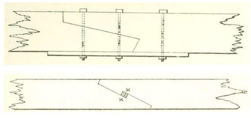
19 C illustration - Joining of timbers, with iron plate and bolts for additional strength
