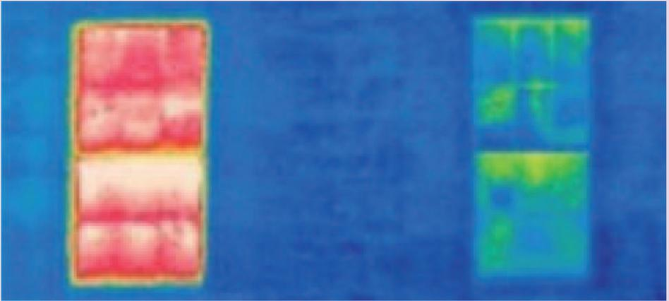
**Fig. 5** Thermal image showing the reduction in heat loss with shutter closed (right) and shutter open (left).
