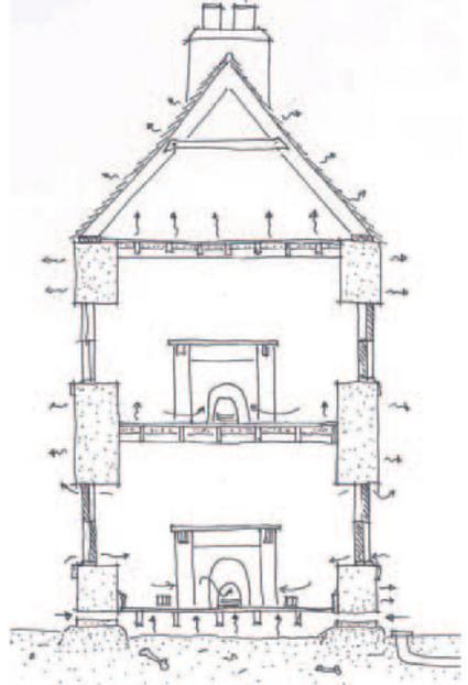
*Fig. 1 Section through a traditionally constructed building showing airflow and vapour movement.*
