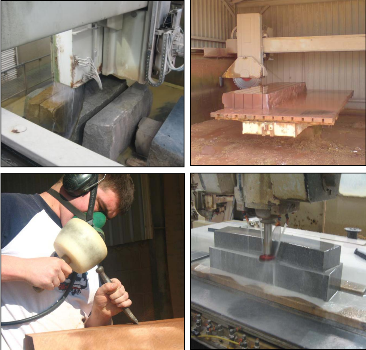
Figure 2: (clockwise from top left) Primary sawing of granite rough block; sandstone block during secondary processing; stone finishing by 3-D profiling machinery; hand finishing.
