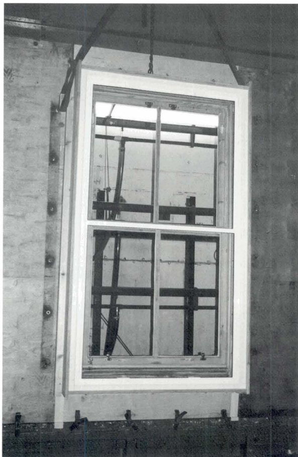
55 Traditional sash and case window undergoing performance tests at Paisley University.
