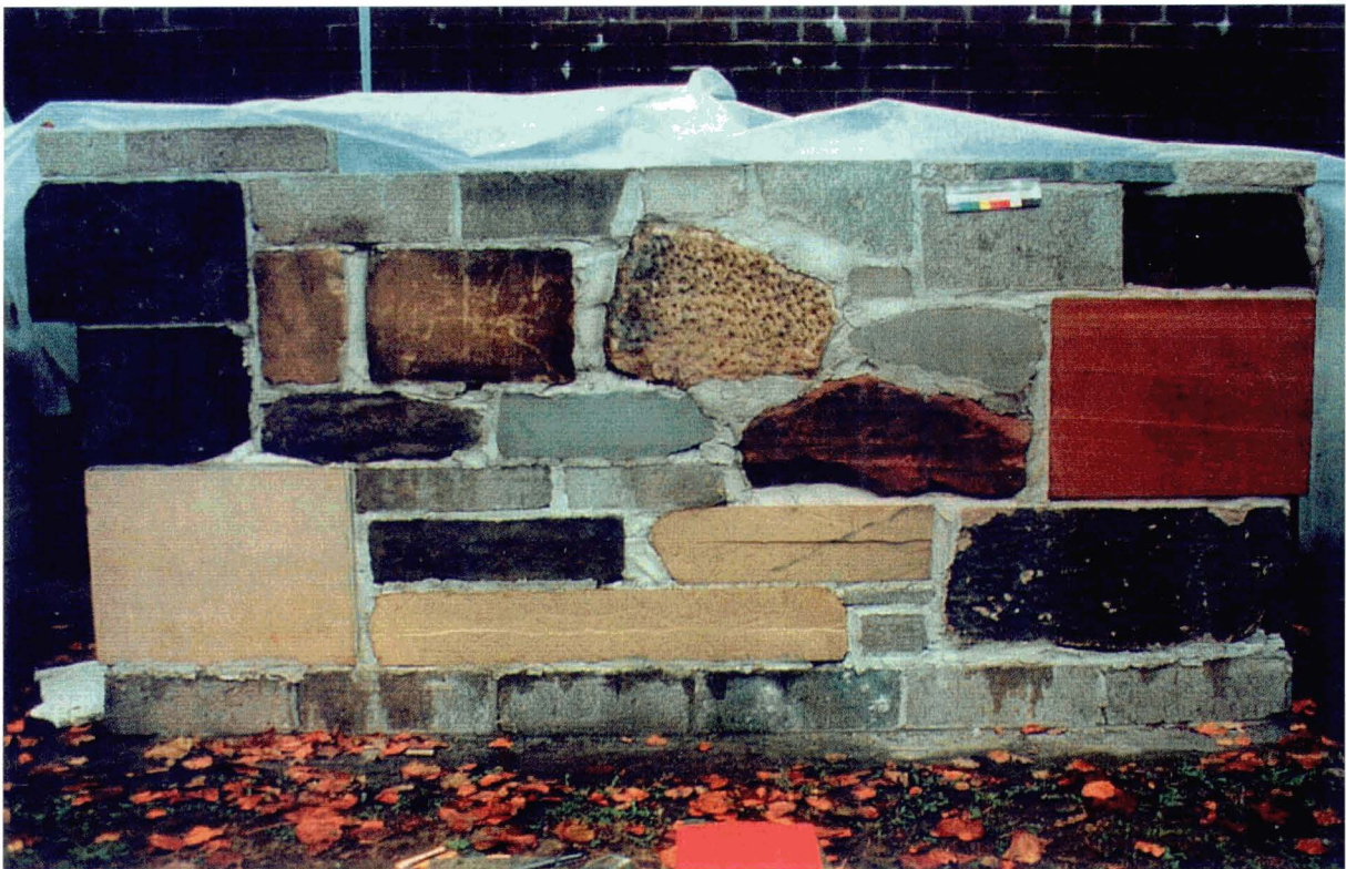
Figure 13i RGU Panel 5. Treated with Consolidant B.
