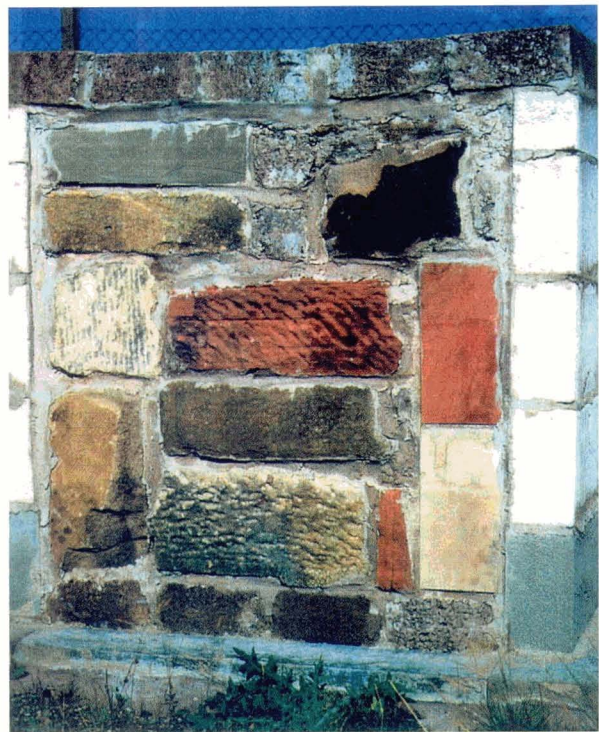
Figure 21 Panel 2 after one year's exposure.
