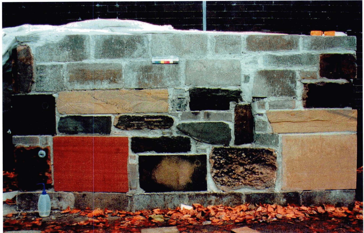
Figure 13c RGU Panel 2. Treated with Consolidant A.
