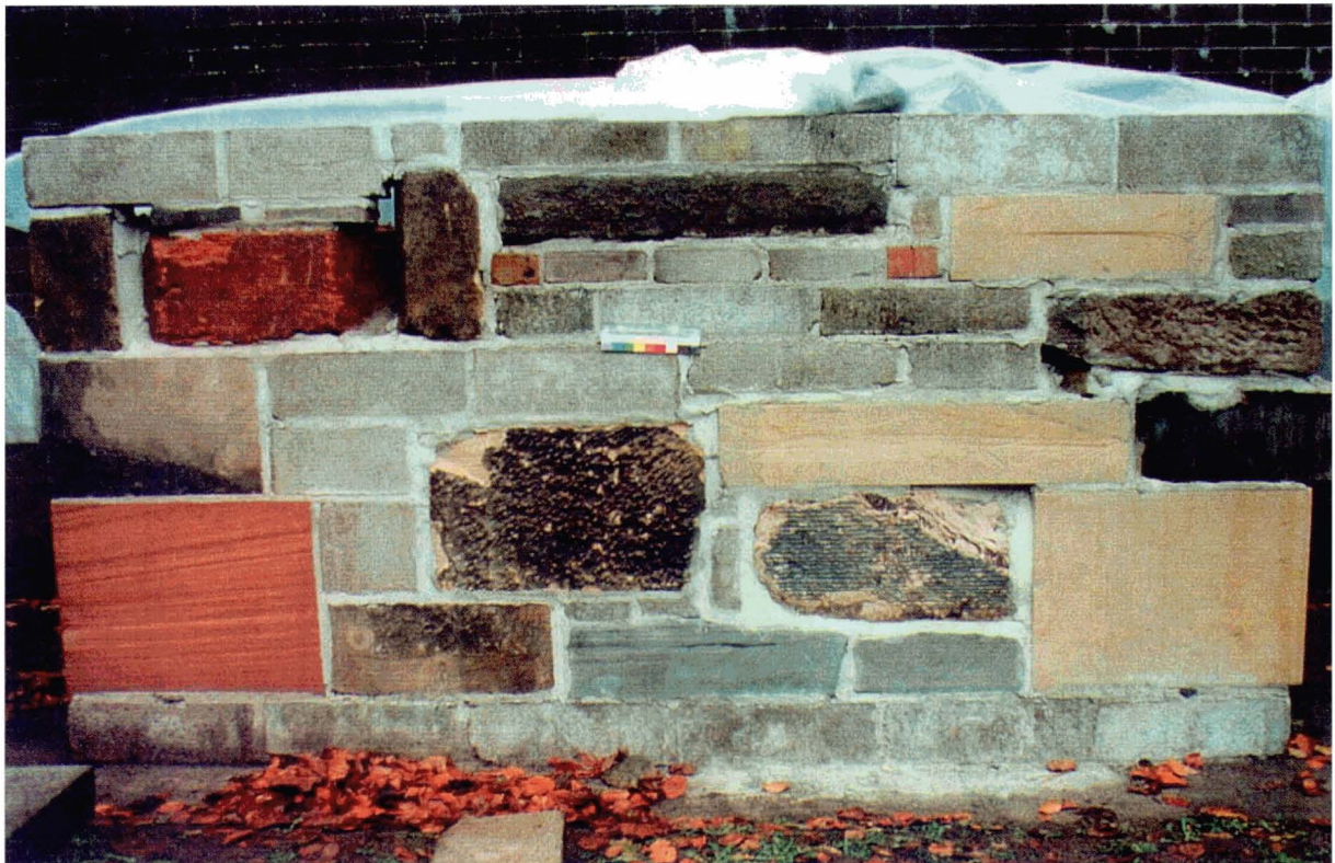
Figure 13e RGU Panel 3. Treated with Water Rep./Con. C.
