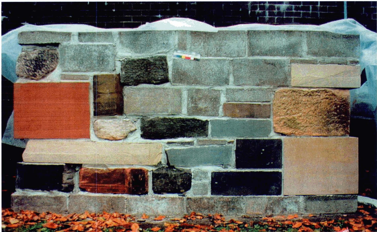
Figure 13g RGU Panel 4. Treated with Water Repellent D.
