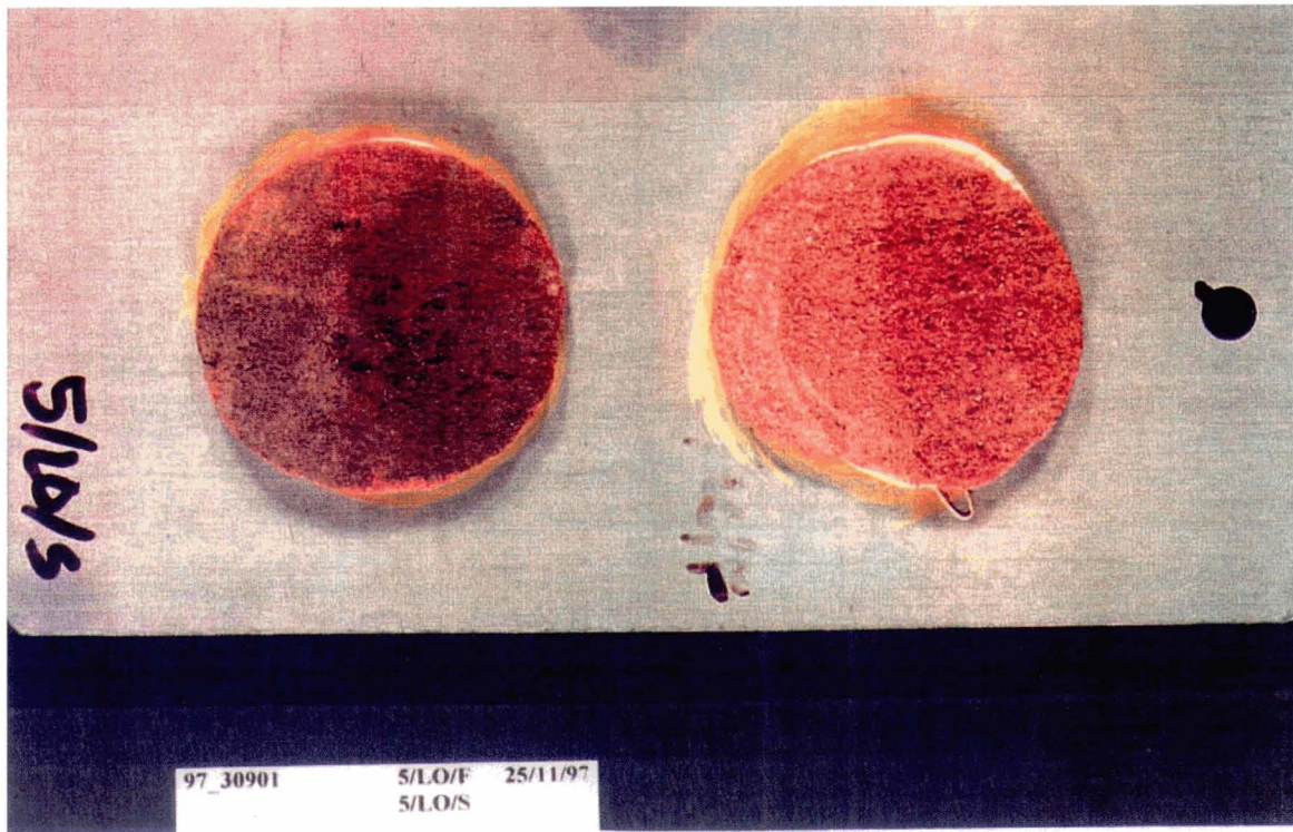
Figure 36c The change in appearance caused by UV-B exposure of Consolidant B treated samples of soiled Locharbriggs (left) and fresh Locharbriggs (right).
