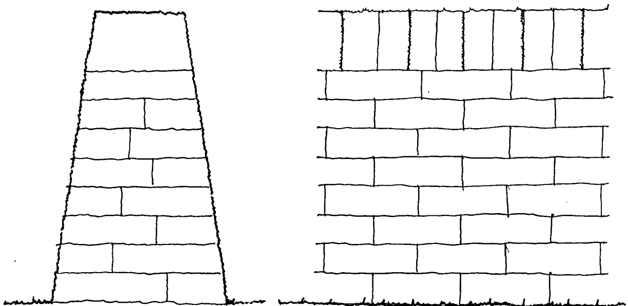
fig 54. Section and elevation of Kailyard Dyke, Burns' Cottage, as preferred by the builder.
