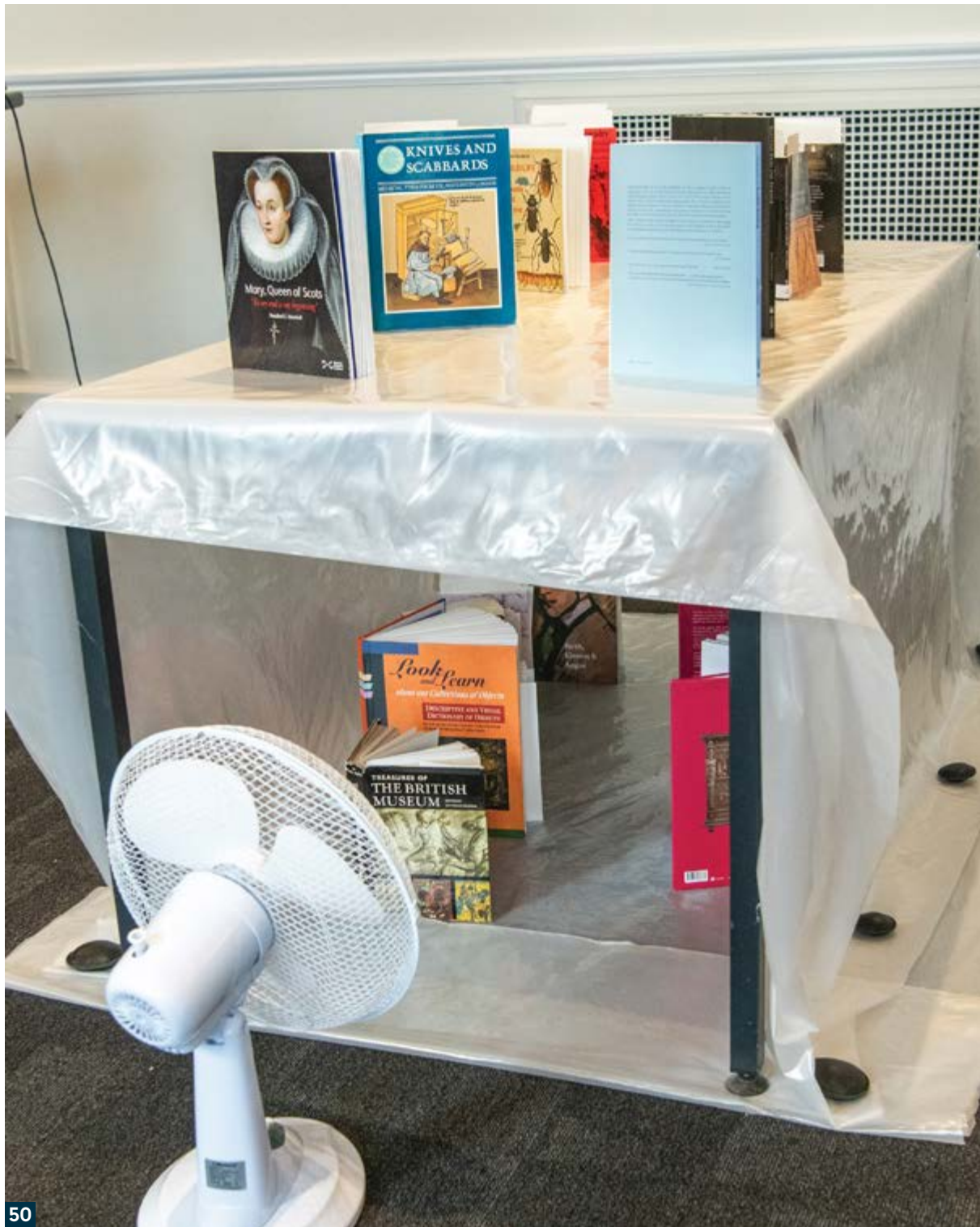
Figure 50. A simple wind tunnel can be constructed to help air dry paper items that have become damp.
