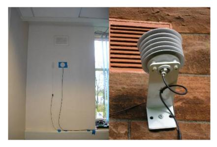
Fig. 2. Monitoring equipment for measuring the U-values of walls before and after the works
