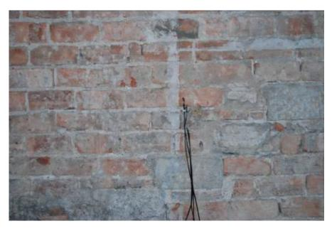
Fig. 8. Probes were set into the masonry to track any changes in humidity levels
