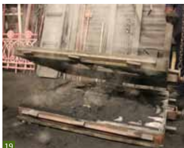
Fig 19 Once the iron has cooled and solidified, the moulding box is opened to remove the casting.
