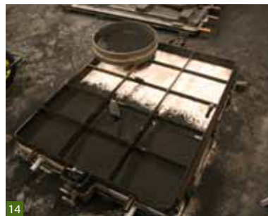
Fig 14 The second half of the moulding box is placed on top and the process of 'ramming' sand is repeated.
