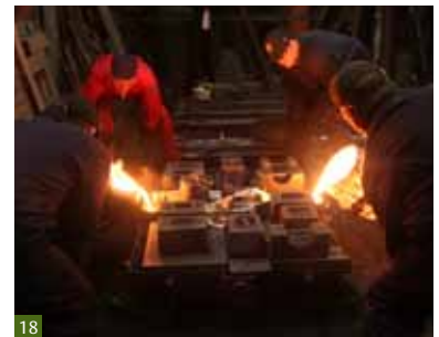
Fig 18 The two halves of the moulding box are put back together again and molten iron is poured into the mould.
