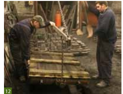
Fig 12 The first half of the moulding box is flipped over so that the underside is now on top.
