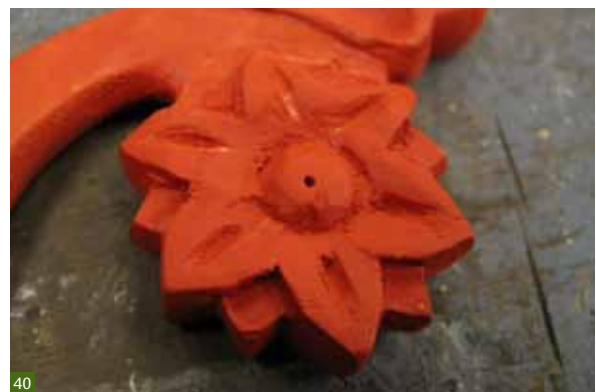
Fig 40 Poorly finished, inaccurate patterns will result in poor quality castings.
