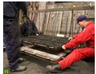
Fig 15 The two halves of the moulding box are separated.
