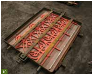
Fig 10 A pattern is placed in one half of a moulding box.
