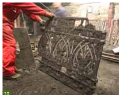
Fig 20 The 'runners' and 'gates' have to be removed in order to finish the casting.
