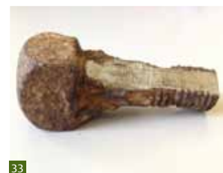
Fig 33 A 19th century iron fixing. The small dark lines of slag (silica) which are visible in the ground-back section of the fixing indicate that it is made of wrought iron.
