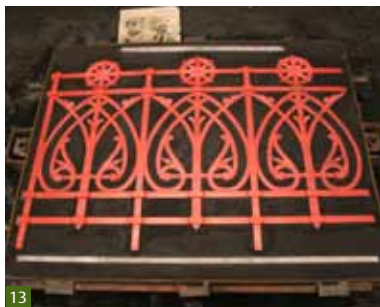
Fig 13 The timber backing board is removed to reveal the underside of the pattern.
