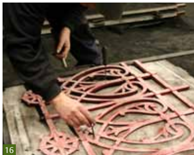
Fig 16 The pattern is removed to leave a void in the sand.
